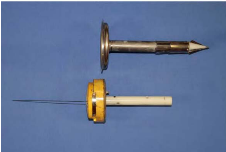
Figure 1. Photo of GPS/TDR tag with yellow syntactic foam float, and the sub-dermal attachment sleeve and protective collar from which it is spring-ejected after a pre-programmed period of time after deployment. The tag will also eject after a predetermined portion of the battery power has been used, or the tag fails to change depth for a predetermined period of time. The latter two circumstances assure that the tag will still have enough energy to determine and transmit its location to facilitate recovery, as well as assure that it floats to the surface should the entire mechanism come off the whale prematurely and sink to the bottom.
