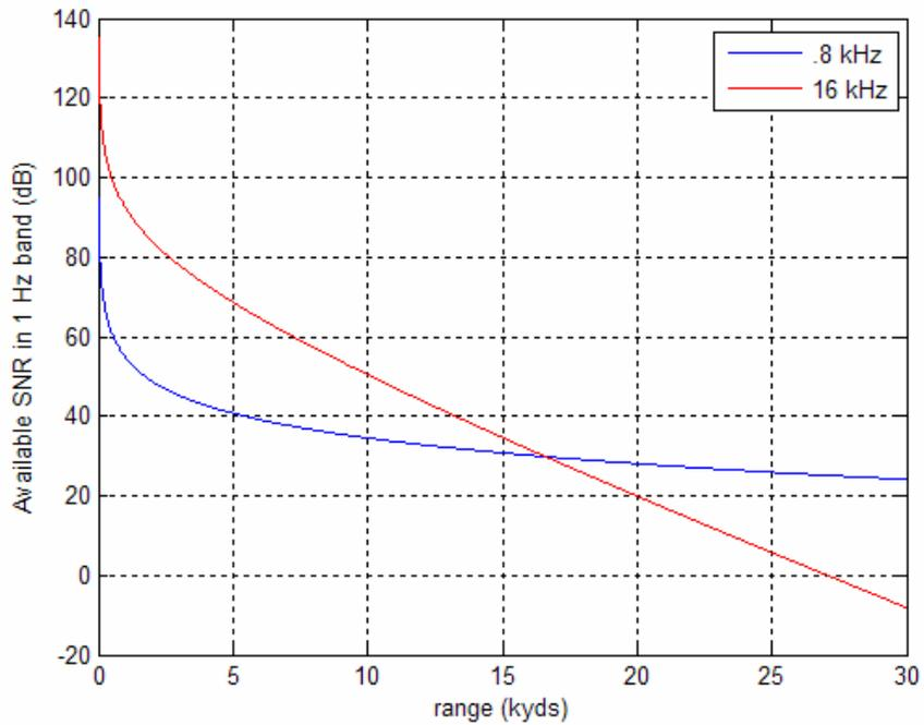
**Figure 3 Detection Thresholds for 8 kHz and 16 kHz.**
