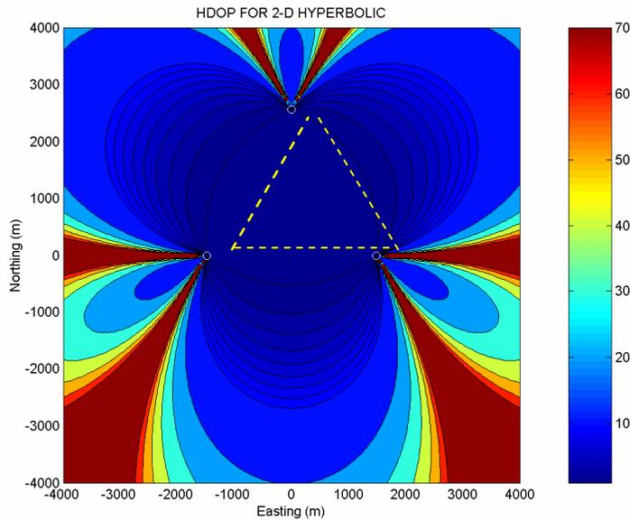
**Figure 7. Equilateral 2-D Hyperbolic Horizontal Geometric Dilution of Precision (GDOP)**
