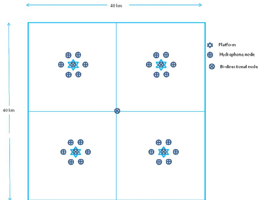
**Figure 8 Post Production Field Node Configuration**
