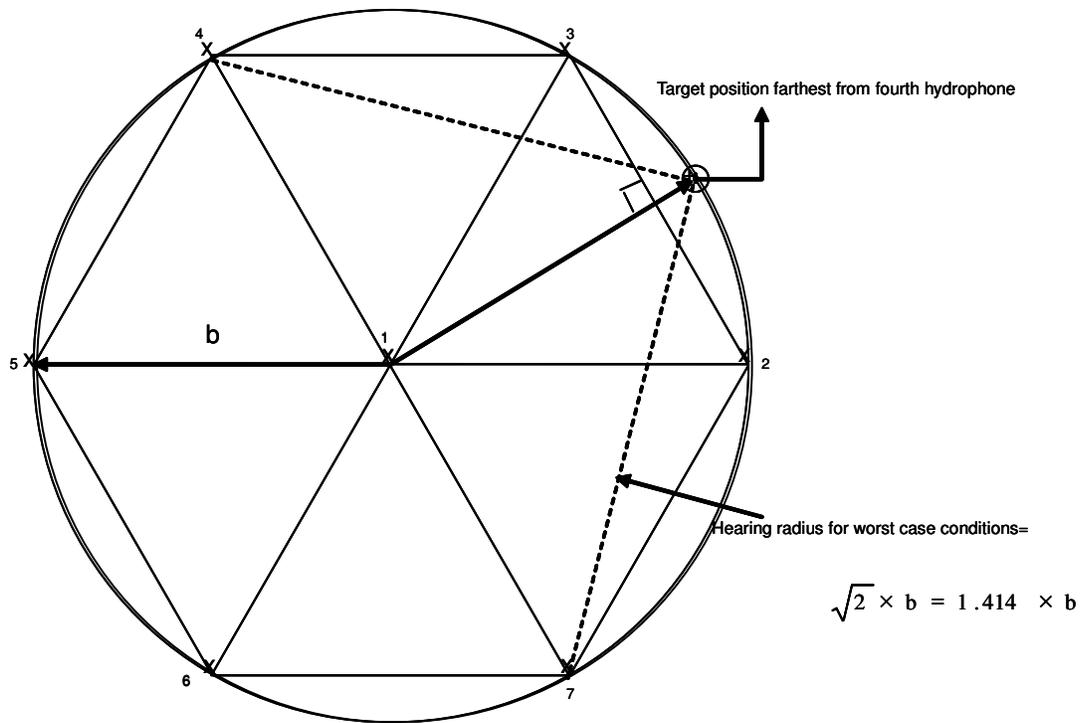
**Figure 8 Hexagonal Array of Receiving Nodes**
