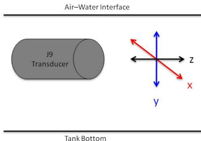
**Figure 16.** Axes considered in tank mapping. The x-axis and y-axis are orthogonal to the longitudinal axis of the J9 while the z-axis is parallel to the longitudinal axis of J9. The air-water interface and tank bottom are also depicted.
