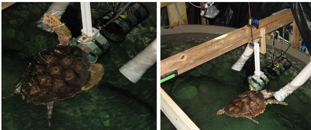
**Figure 7.** Freely swimming turtles enter observer ring positioning themselves head on relative to the J9 and equidistant from the response chutes (left). A white light above the tank is triggered to signal trial onset, initiating acoustic presentation and video recording. The turtle indicates a response by biting either a 'no signal' or 'signal' chute (right).
