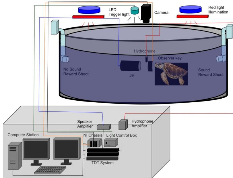
**Figure 6.** Schematic of data acquisition and stimulus delivery (DASD) system used for behavioral trials for the Cc2005 year class of turtles. The items in the gray box were set up in a separate room from the experimental tank so that turtles were not influenced by researchers.
