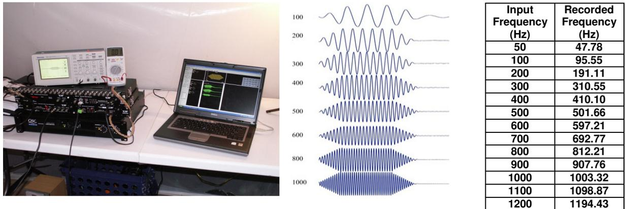
**Figure 5.** TDT system (left), example of tone burst stimuli (middle), and input and actual recorded frequencies (right) produced using TDT system for behavioral audiogram experiments.
