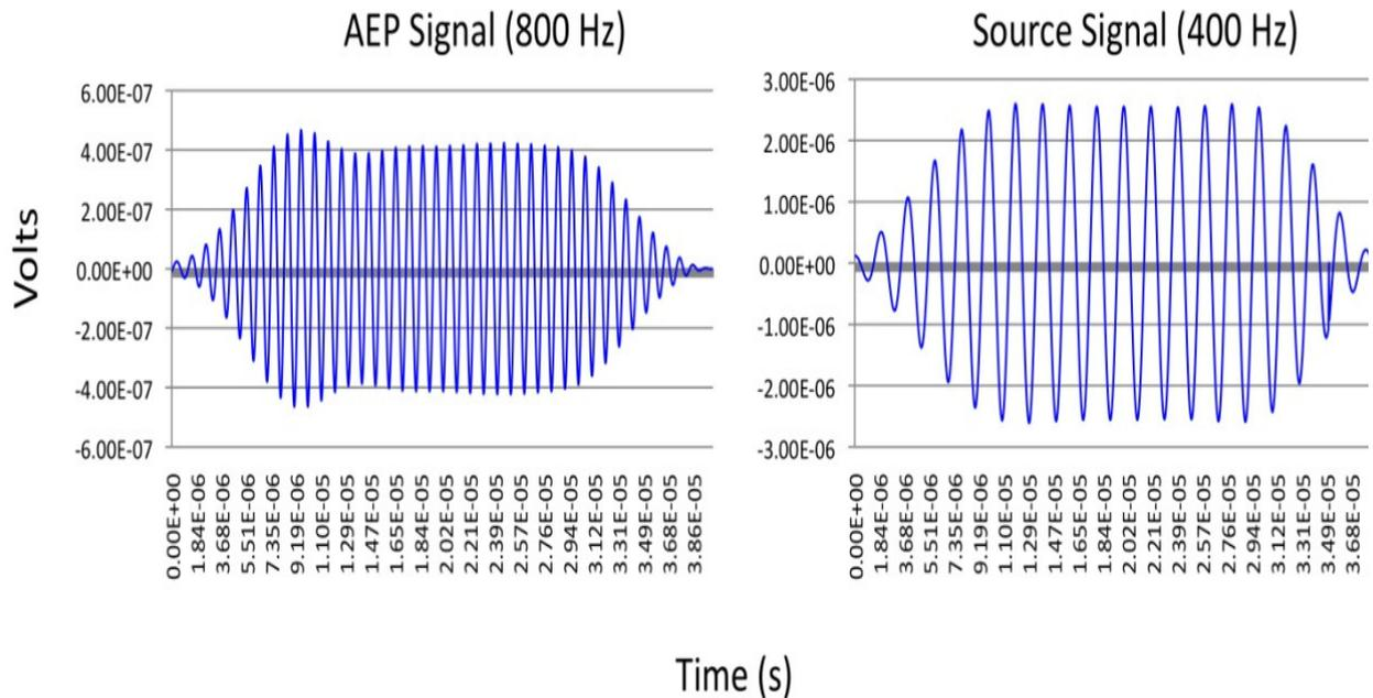
**Figure 11.** Example of AEP signal (left) recorded from a source signal (right) of 400 Hz. Note that the AEP signal is twice the frequency of the source signal, which is a result of simultaneous responses from two groups of hair cells oriented in opposite directions.
