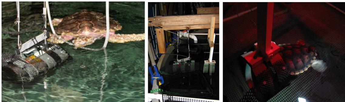
**Figure 4.** Initial trigger used for behavioral training involving a reinforced tube with an integrated pressure transducer (left) and the revised trigger consisting of a plastic ring that triggered light and sound delivery when the turtle inserted its head into the ring structure (middle and right).
