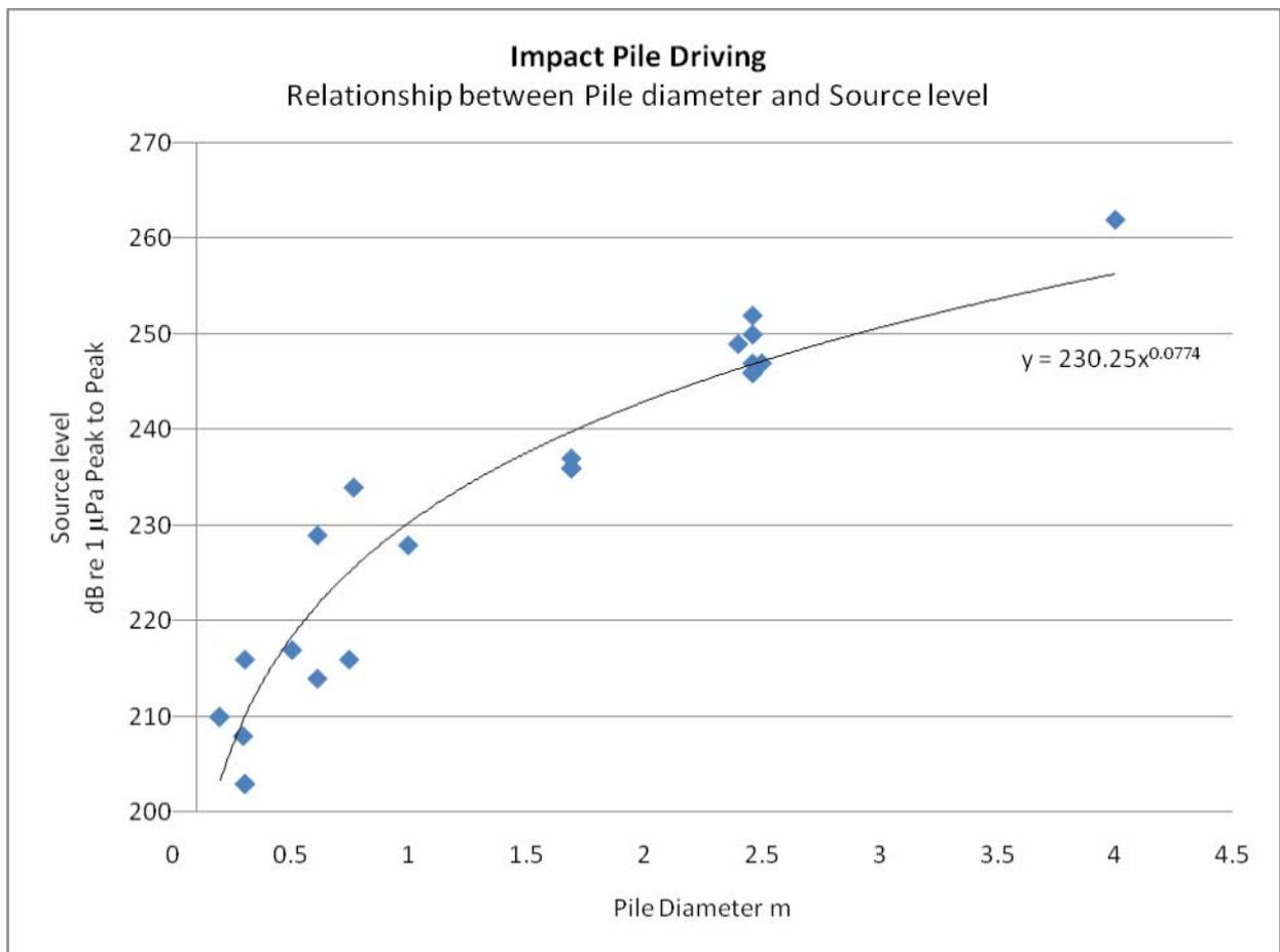
Figure 3.3. The relationship between pile diameter and peak to peak sound pressure level ( $x$  is the pile diameter in metres and  $y$  is the peak to peak sound pressure)
