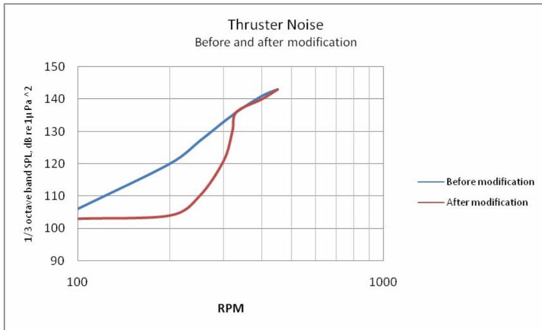
Figure 3.18 Thruster Noise showing onset of cavitation at around 250 RPM (Brown, Dai et al. 2001)
