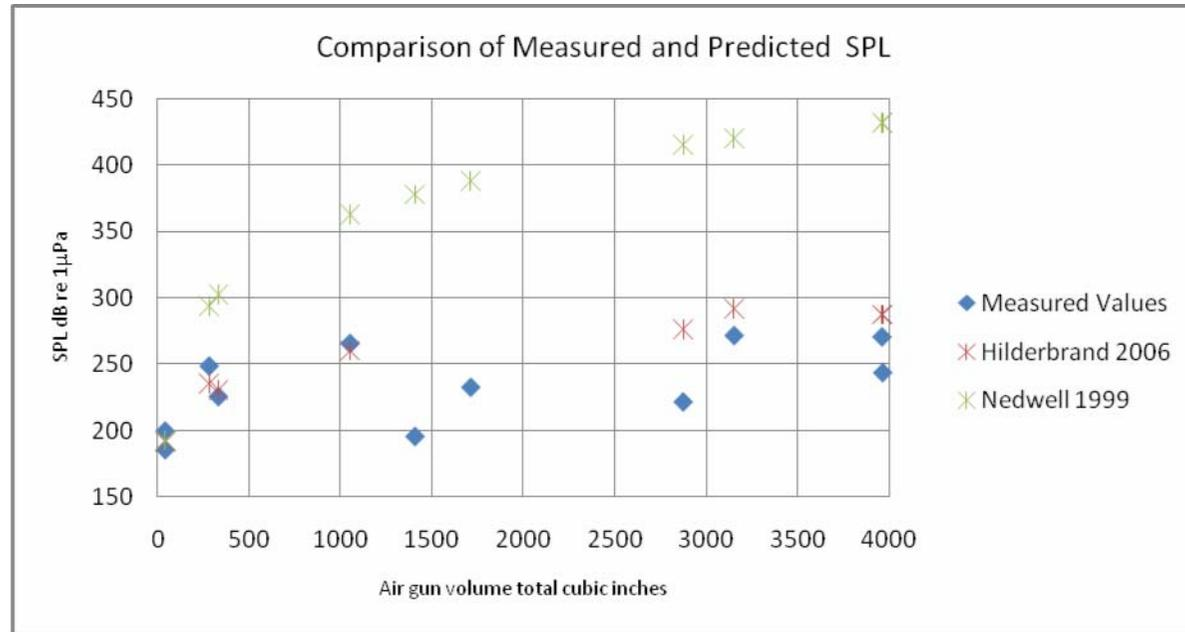
Figure 3.14 Comparison of measured and calculated air gun SPL.
