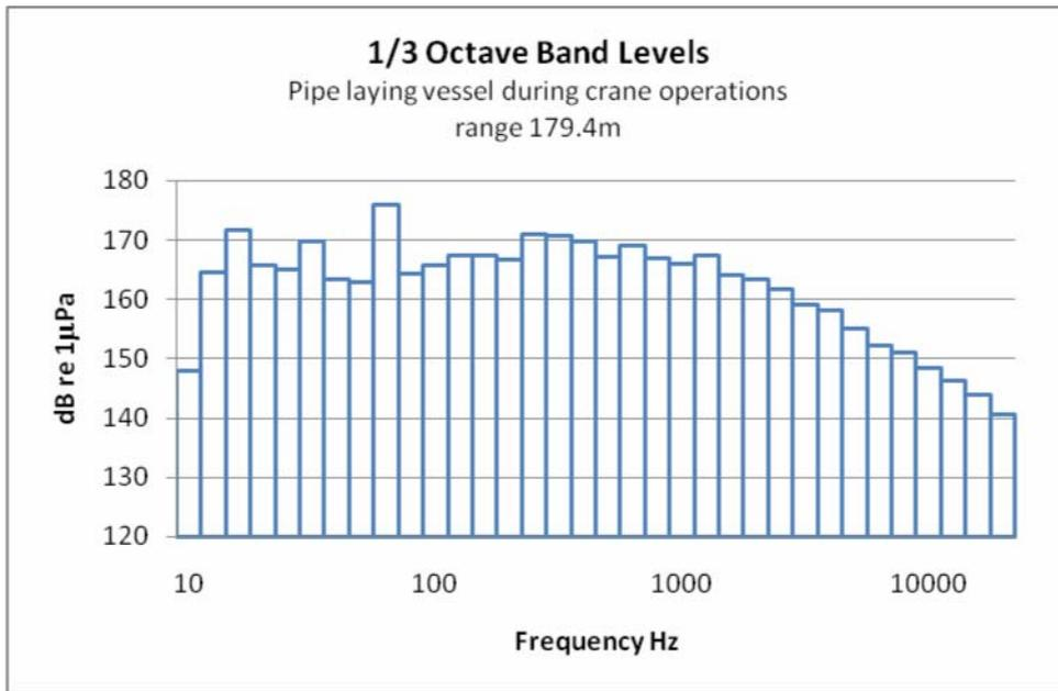
Figure 3.6 Third octave band analysis of pipe laying barge during crane operation (MacGillivray and Racca 2006)
