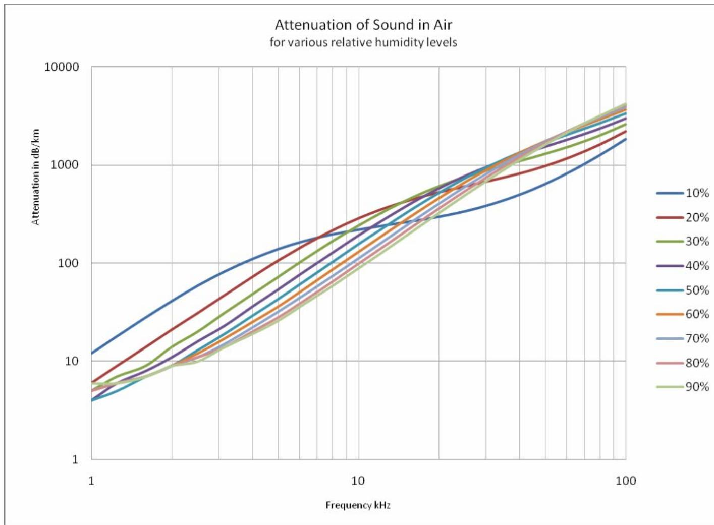
Figure B.7 Sound transmission through air adapted from (Kaye and Laby 1986)
