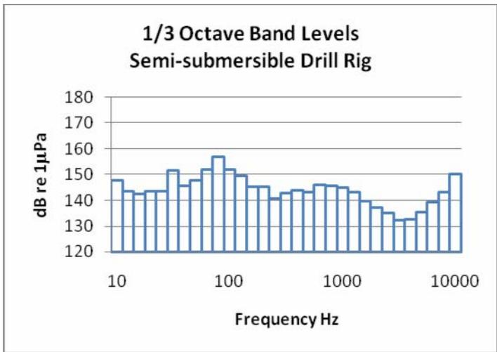
Figure 3.12 Third octave band levels for semi-submersible drill rig
