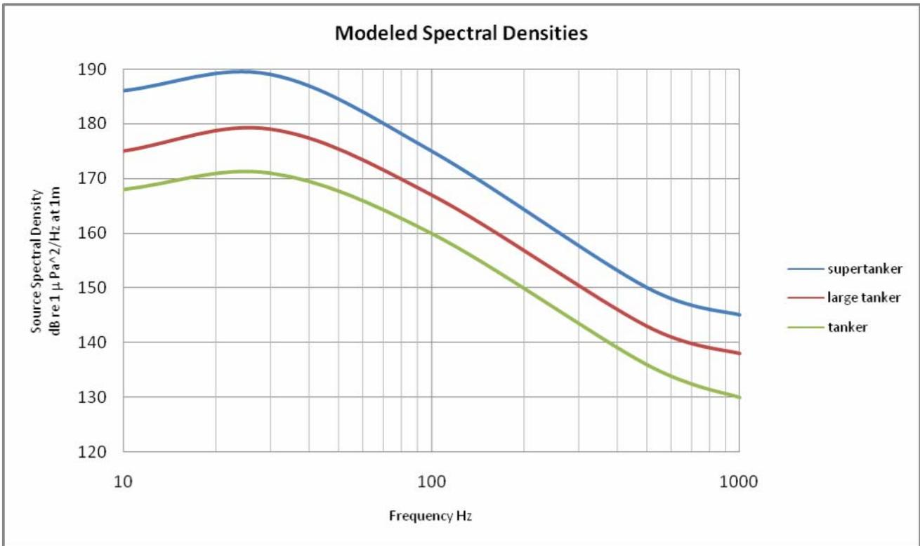
Figure 3.16 Modelled spectral densities of a range of tanker sizes
