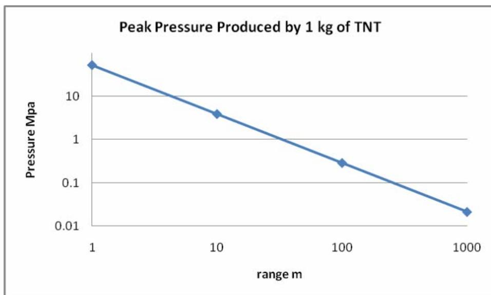
Figure 3.13 Peak pressure produced by 1Kg of TNT
