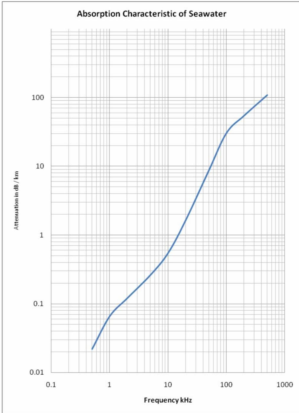
Figure B.5 Sound attenuation properties of seawater adapted from Urick (Urick 1967)
