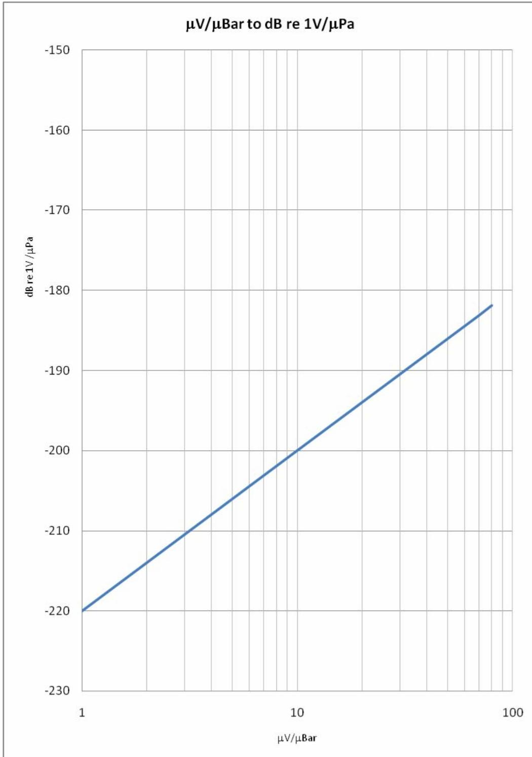
Figure B.3 Sound pressure level conversion  $\mu\text{V}/\mu\text{Bar}$  to  $\text{dB re } 1\text{V}/\mu\text{Pa}$
