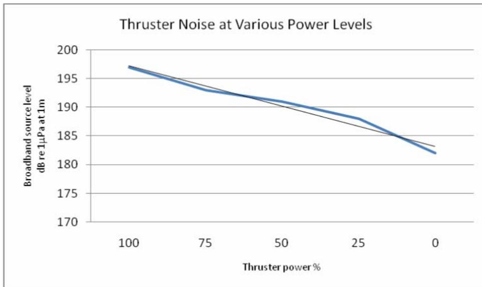
Figure 3.17 Thruster noise. Adapted from (Austin 2005)
