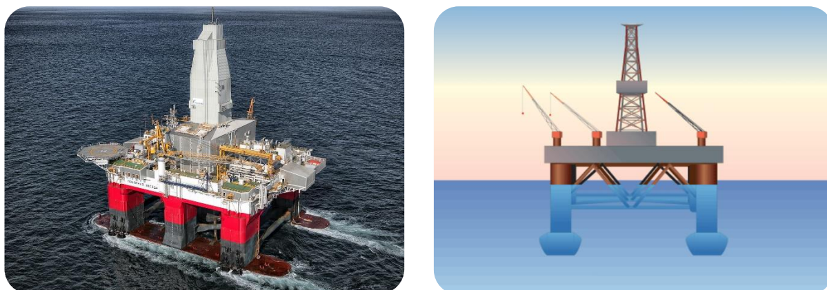
Figure 5.21 Self-propeller semi-submersible drilling rig MOSS CS-50 Mk II Polyarnaya Zvezda (left, from www.oaoosk.ru ) and diagram of a deep-water semi-submersible (right, from www.glossary.oilfield.slb.com )
