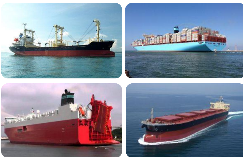
Figure 4.5 Types of dry cargo vessels, from left to right and top to bottom: general cargo vessel, container vessel, RO-RO vessel and bulk carrier (from www.tuscorlloyds.com )
