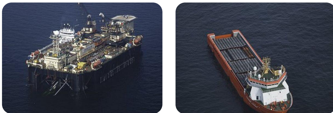
Figure 5.31 Photo of pipe-lay vessel Castoro Sei (left) and pipe-carrier Normand Flipper (right). From Johansson & Andersson (2012).
