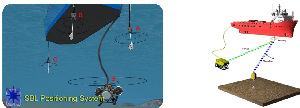
Figure 3.12 Configuration of hull-mounted Short Baseline (left, from www.desertstar.com ) and Ultra-Short Baseline (right) positioning systems. In the left image, A,C,D are the surface transceivers and B the transponder mounted on the tracked object.
