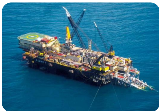
Figure 5.33 S-lay barge SEMAC-1 (left, from www.drillingformulas.com ) and J-lay barge (right, from www.rigzone.com )
