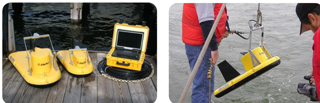
Figure 3.6 Chirp sub-bottom profiling system 3100, with towfish SB-216S and SB-424 (left) and deployment detail (right). From www.edgetech.com .
