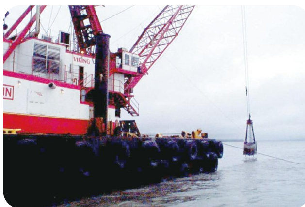
Figure 5.9 Grab dredge Viking operating in Cook Inlet, Alaska (from Dickerson et al., 2001).
