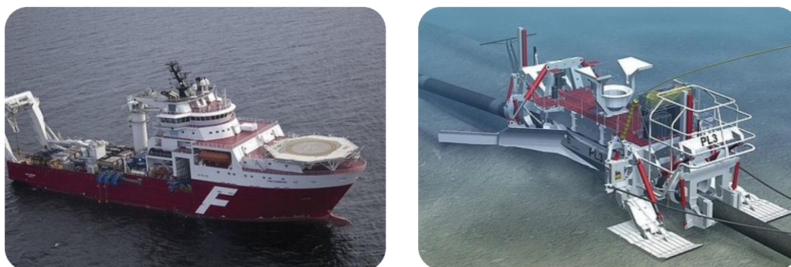
Figure 5.32 Photo of post-lay trenching vessel Far Samson (left) and sketch of post-lay trenching plough (right). From Johansson & Andersson (2012).
