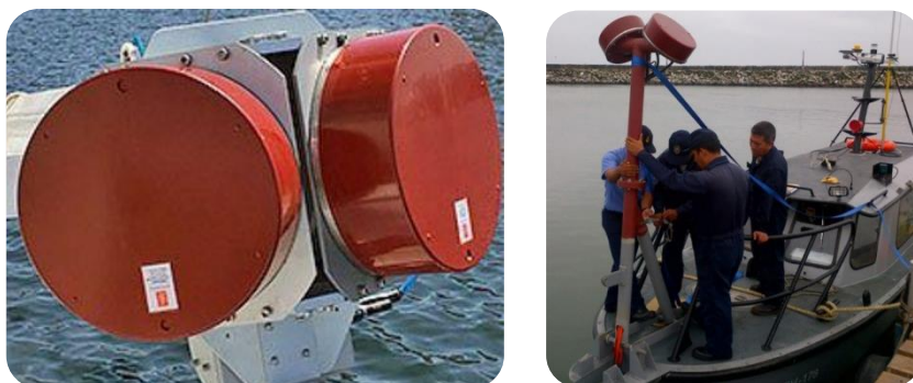
Figure 3.2 Multi-beam echo sounder EM 2040C (left) and bow mounting detail (right). From www.km.kongsberg.com
