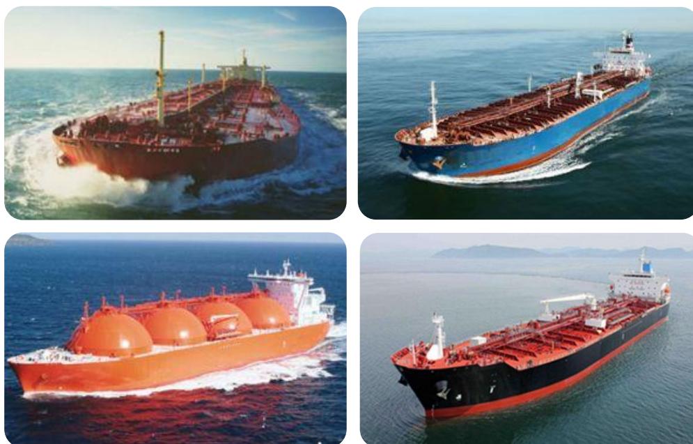
Figure 4.6 Types of liquid cargo vessels, from left to right and top to bottom: crude oil tanker, product carrier, liquefied gas carrier and chemical carrier (from www.tuscorlloyds.com )
