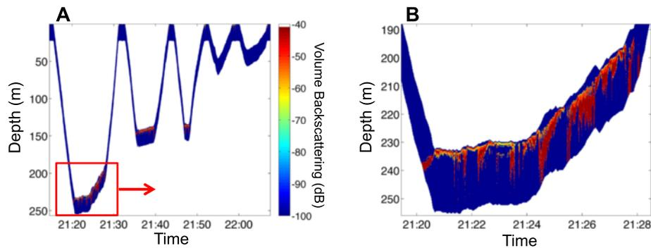
**Fig. 4** Sonar tag acoustic data showing evidence of bottom scattering. **a** One hour subset of acoustic data associated with translocated seal #4. Strong bottom scattering associated with benthic-type dives is evident as the animal moved toward shore off the Monterey Peninsula (region 1 in Fig. 2). **b** Zoom in on bottom-associated scattering
