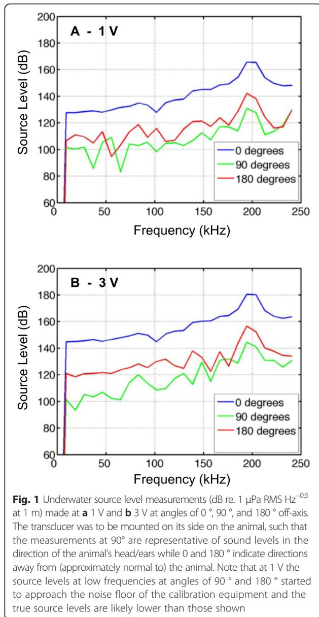
(re.  $1 \mu\text{Pa RMS Hz}^{-0.5}$  at 1 m), respectively. The goal of the source level calibrations relative to frequency was to determine operational voltages for which the source level would be as low and as close to inaudible to the seal as possible in its hearing band while also maintaining reasonable signal-to-noise ratios (SNR). The upper frequency cutoff for northern elephant seal hearing in
