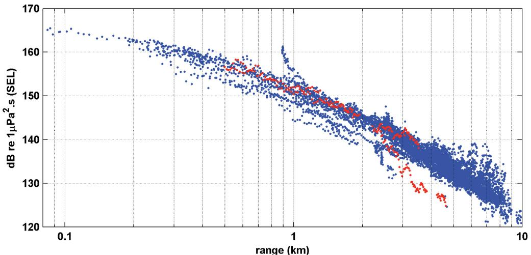
**Figure 2.** Decay curves of measured 20 cu in air gun SEL with log range; multiple air gun runs and multiple propagation paths are overlaid, and much of the spread in points is due to the differences between runs and paths. The blue curves are multiple runs across sand only; the red curve is one air gun run across the high loss rate rock from greater than 2.36 km on one leg.
