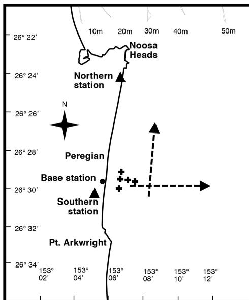
**Figure 1.** The Peregian study area. The hydrophone buoy array is indicated by crosses, while the two transects of the source vessel, eastwards and northwards, are indicated by the dashed arrows. The land-based observation stations are shown by the triangles.
