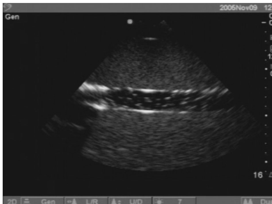
Fig. 2. Ultrasound image of small bubbles flowing through the tissue and vessel phantom. The bright spots within the vessel are bubbles.
