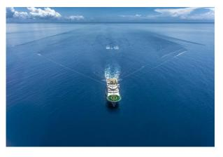
A vessel towing a seismic array
