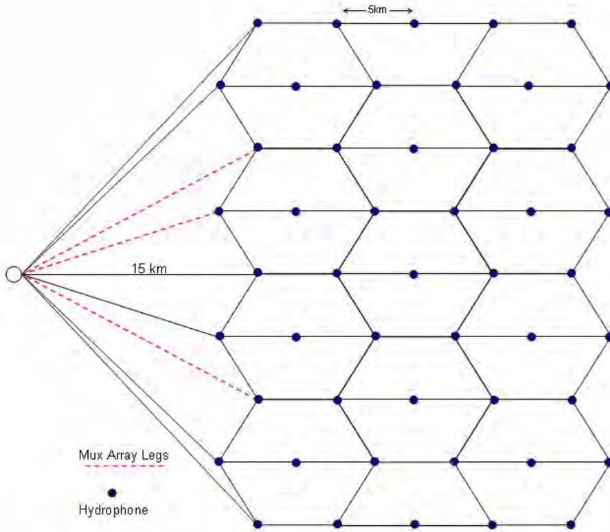
**Figure 9. Idealized Range Layout for ~1000 km area with 5 km sensor baseline**
