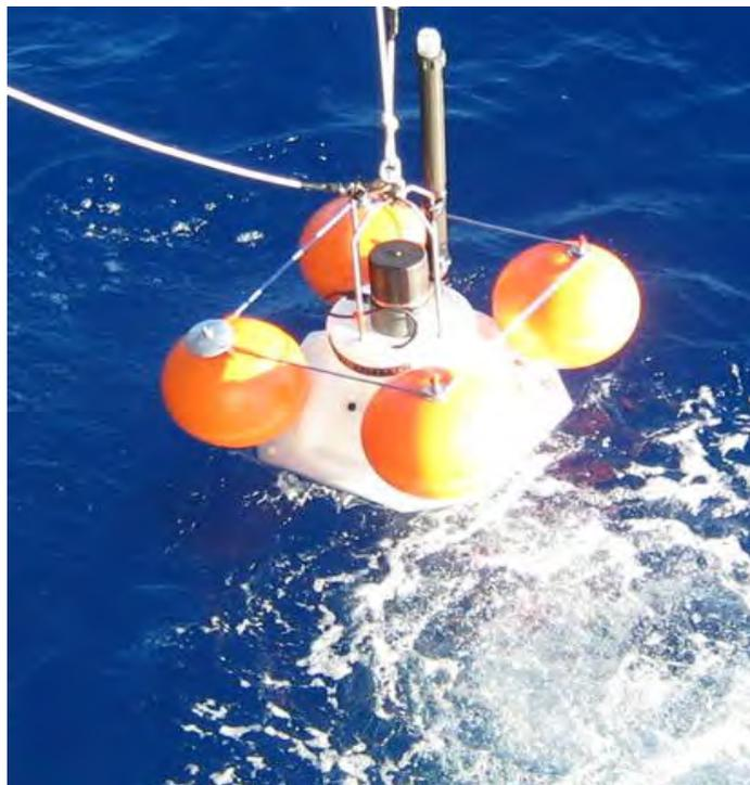
Figure 10. MIKEL Inc. Dual use Recording Smart Transponder/Beacon
