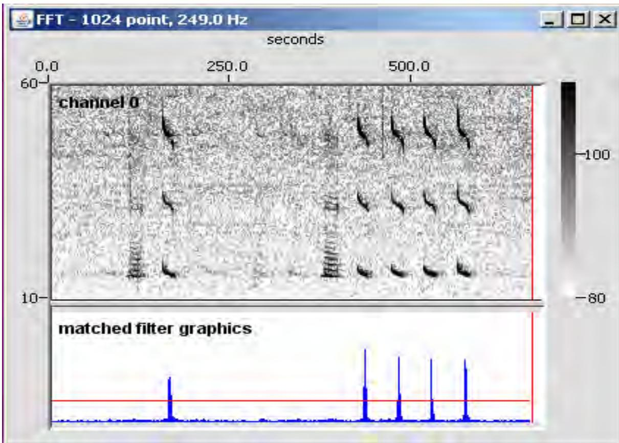
**Figure 10. Example of a detection threshold used in detection of blue whale calls. The detection threshold is the red line in the lower panel; any time the detection function (blue) exceeds this threshold, a detection is registered. From [28].**
