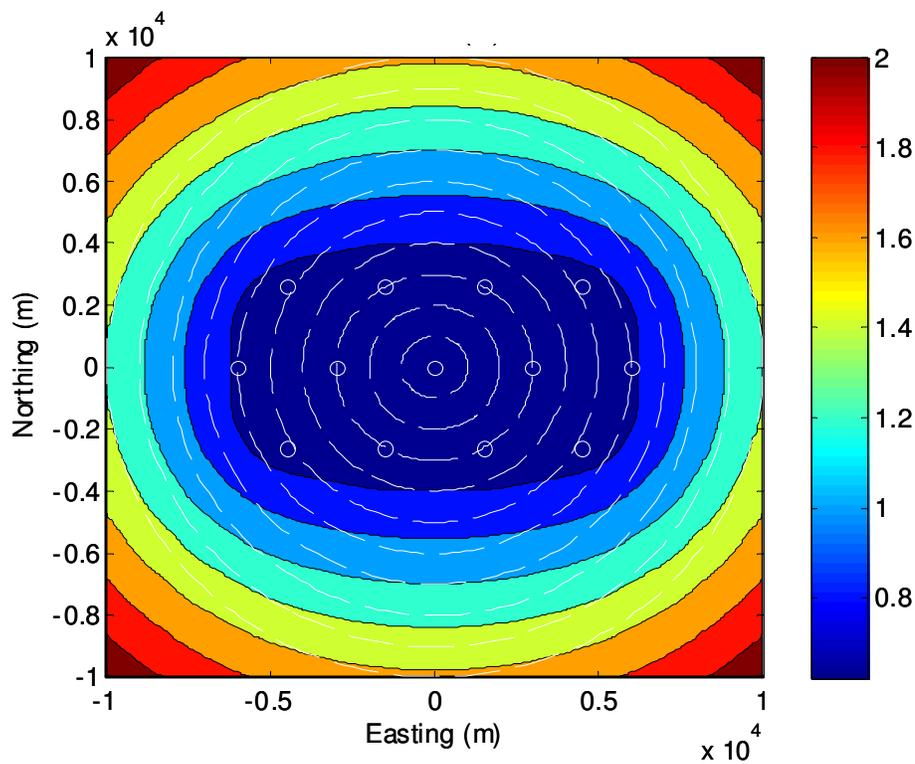
**Figure 9 GDOP for Expanded Hyperbolic Tracking Array**
