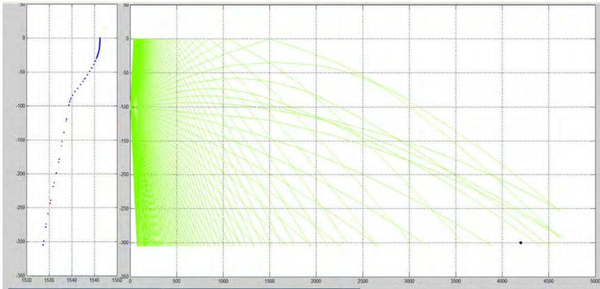
**Figure 7. SVP and raytrace for downward refracting environment with source at 100m depth and bottom-mounted hydrophone at 4.2 km distance in 300 m water depth.**
