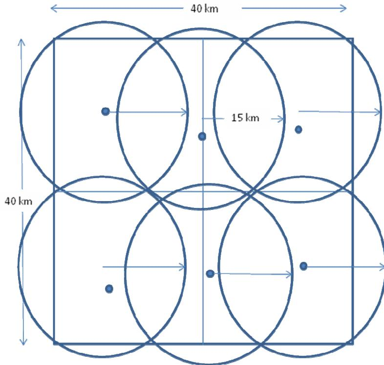
**Figure 5. Multi-Node Area of Coverage**
