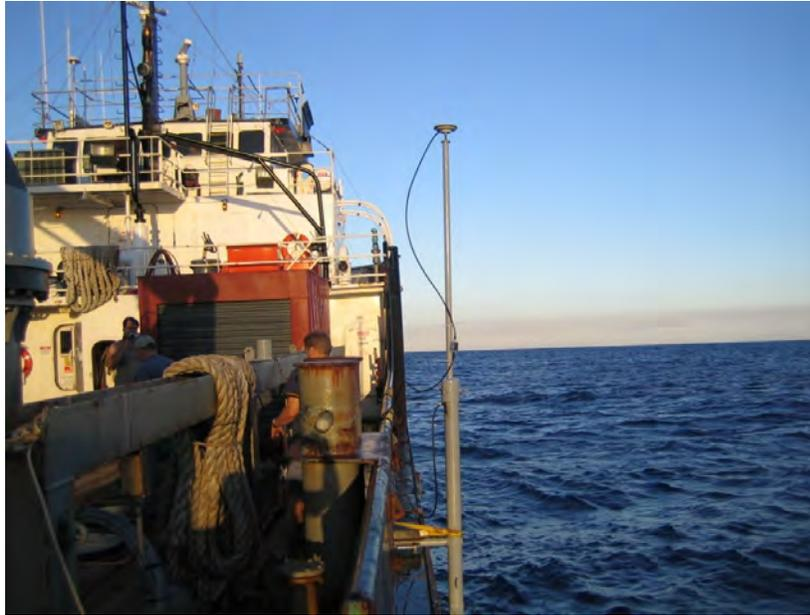
**Figure 11 Pinger Pole with GPS**
